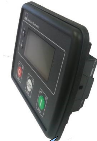
Gasket fitted to module
